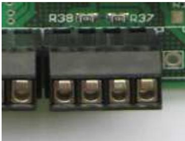
GND, one wire bus 1, one wire bus 2, +5V
